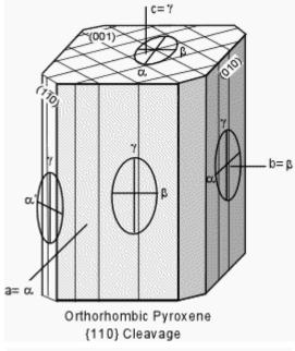
In Cpx, however, one would see inclined extinction on all faces except {100}. Thus, one should check several grains for extinction before concluding that the mineral is Opx, since there is always a slight chance that one is looking at a {100} face. Note that in Cpx, the maximum extinction angle will only be observed if one is looking at a {010} face.
