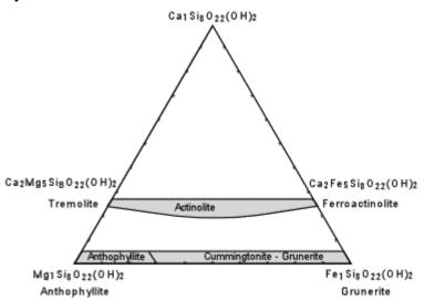
Hornblende is the most common amphibole and has more in common with the Tremolite - Ferroactinolite series, with Al substituting into the Y sites and the tetrahedral site. It thus has the complicated formula:
