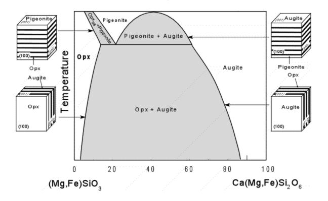
When pigeonite or augite exsolve they may form exsolution lamellae that form parallel to the (001) plane. At lower temperature the exsolution of Opx or augite result in exsolution lamellae that are parallel to the (100) plane.
