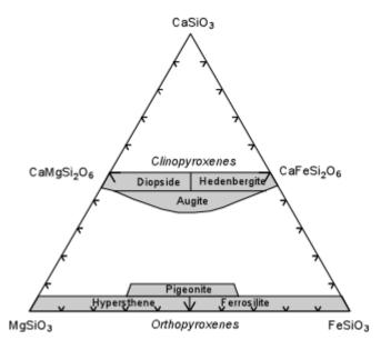
There is complete Mg-Fe solid solution between the pyroxenes, and as with most Mg-Fe solid solutions, the Mg-rich end members crystallize at higher temperatures than the Fe-rich end members.
