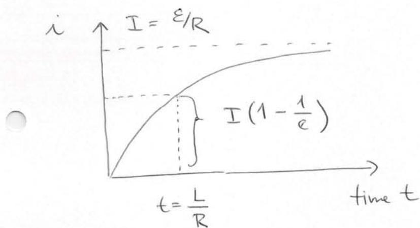
→ for  $t \rightarrow \infty$ , inductor behaves as a simple conducting element with zero resistance
