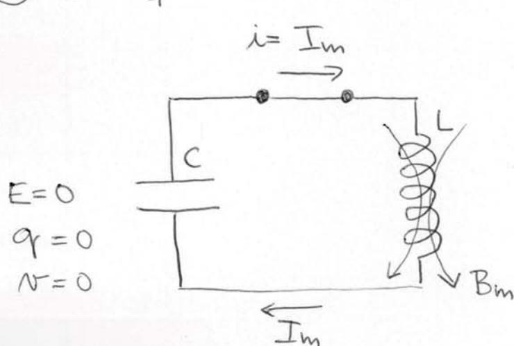
At time  $t = \frac{T}{4}$ , capacitor is fully discharged
