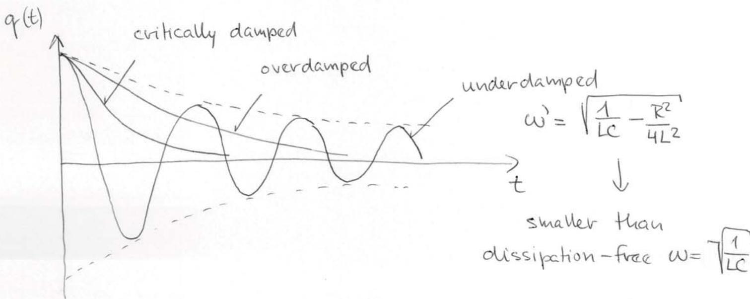
Ex 30.11: Underdamped L-R-C series circuit
