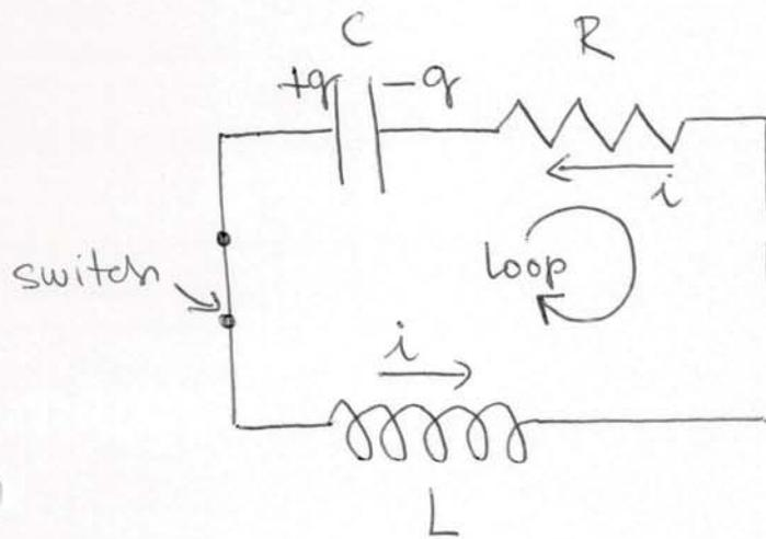
At time  $t=0$ , capacitor is fully charged to charge  $Q = E \cdot C$
