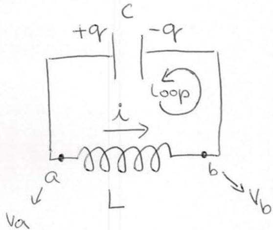
Consider a circuit containing an (ideal) inductor and capacitor
