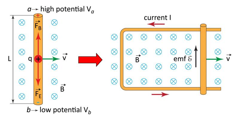
Magnetic force  $\vec{F}_R$  causes charge separation  $\rightarrow$  generation of electric field  $E = (V_a - V_b)/L$  and electric force  $\vec{F_E}$  opposing the magnetic force
