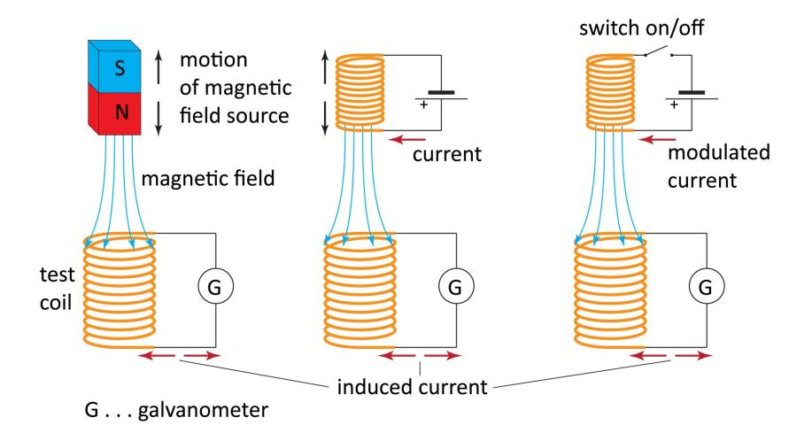
Changing magnetic flux through a test coil leads to generation of induced current through the coil  $\rightarrow$  electromagnetic induction
