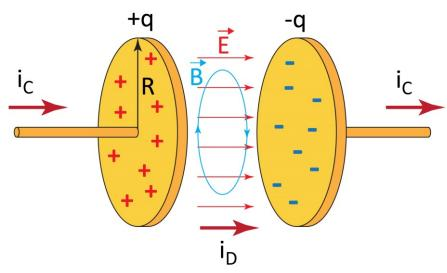
Time-varying conduction current  $i_c$  charging a capacitor is related to the electric flux between the capacitor plates:
