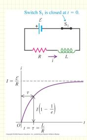
• The rate at which the source delivers energy to the circuit is  $P_{\mathcal{E}} = \mathcal{E}i$ .
