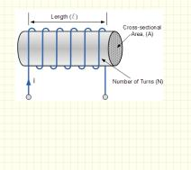
• Prototype of inductors. • n = N/l•  $B = \mu_0 ni$ •  $\Phi_B = BA = \mu_0 niA$ • Then  $L = \frac{M\Phi_B}{i} = \mu$
