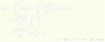
Energy stored in a toroidal solenoid • Recall  $L = \frac{N\Phi}{i} = \frac{\mu_0 N^2 h}{2\pi} \ln \frac{b}{a}$  and so  $U = \frac{1}{2}Li^2 = \frac{\mu_0 N^2 h}{4\pi} \ln \frac{b}{a}i^2$
