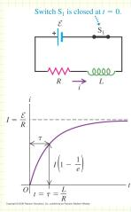
Since the current does not go to zero, there is always some dissipation of energy on the resistor which is supplied by the source.
