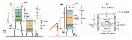
**Fig. 12.3** Schematic detail of construction and operation of a (**a**) split-column unit and (**b**) single unit used in the field, (**c**) details of the coarse sand filter for entrapment of waste backwash containing hydrated ferric oxide particles. (Sarkar et al., 2007)
