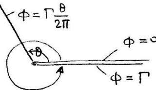
Complex velocity potential which represents the flow due to a vortex located at  $z=z_0$  can then be defined as:
