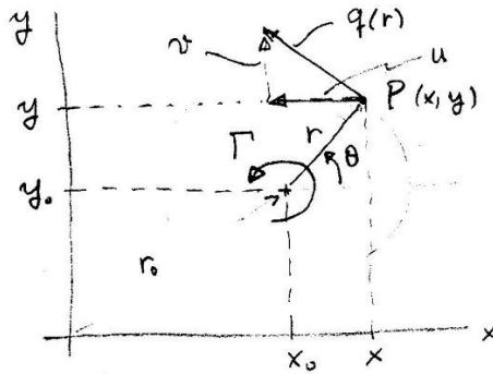
Vortex at point  $(x_0, y_0)$  with strength  $\Gamma$  induces a circumferential velocity field  $q(r)$ .
