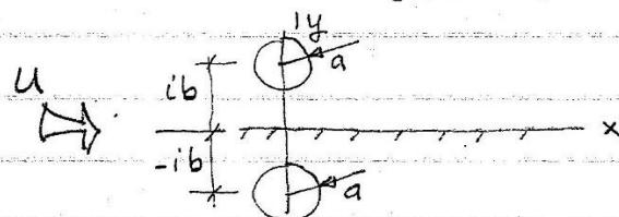
Note that due to the interaction of the doublets, the geometry of the cylinders are distorted a little bit.
