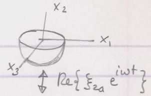
$$(m_{22} + a_{22}) \ddot{\xi}_2(t) + b_{22} \dot{\xi}_2(t) + c_{22} \xi_2(t) = \text{Re}\{A e^{i\omega t}\}$$
