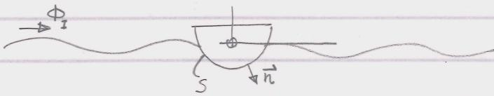
$$\Phi_I = \frac{q \xi_0}{\omega} \frac{\cosh k_0 z}{\cosh k_0 d} e^{i(k_0 x - \omega t)} = \varphi_I(x, y, z) e^{-i\omega t}$$
