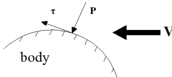
The tangential shear stress ends up with frictional resistance on the body. This force component may be approximated by 2-dimensional flat-plate friction. But one should be aware of the fact that 3-dimensional effect is excluded in this case. Integration of normal stresses due to viscosity over the wetted surface of the body gives the viscous pressure resistance. Cross-flows, vortex shedding and flow separation are the main causes of the viscous pressure drag.
