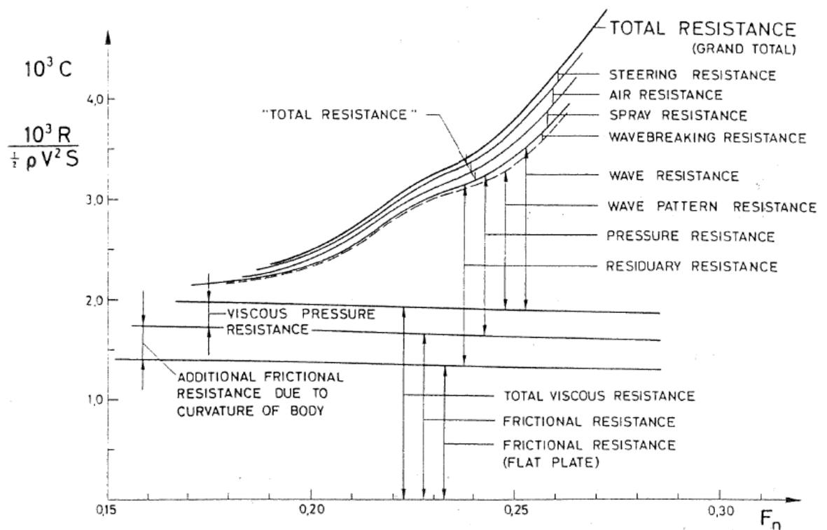
Fig. 3.2: Reduction of total resistance into components (Harvald, 1991)
