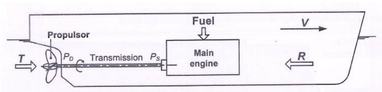
**Fig. 1.1:** Basic elements in the powering of ships (Molland et. al. 2011)
