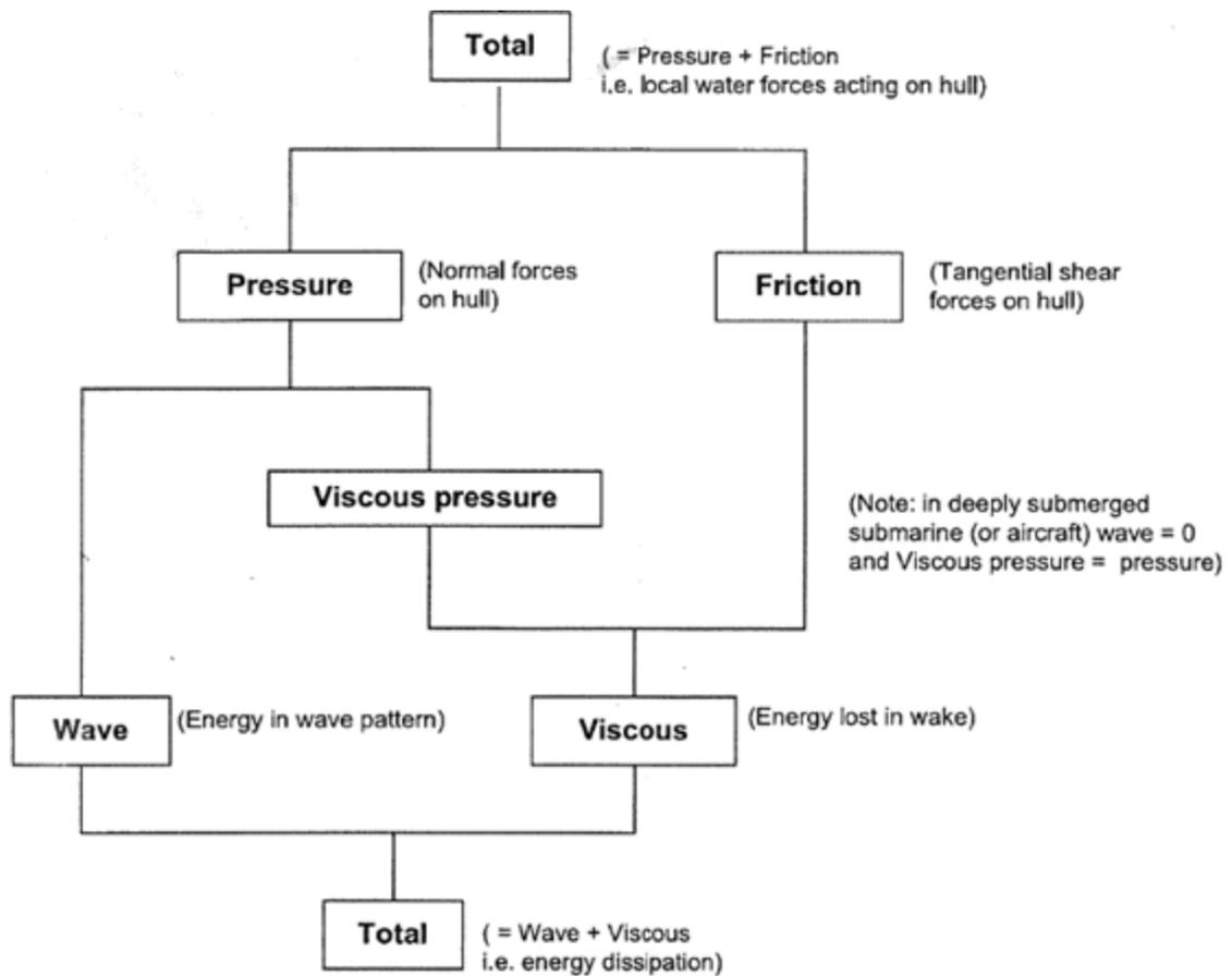
Fig. 3.1: Basic resistance components (Molland et. al. 2011)
