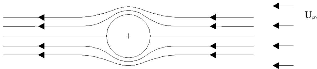
according to *Bernoulli's equation*: the velocity speeds up where the pressure drops and vice versa. Now, if we think this 2D circular cylinder is placed under the free surface, the pressure distribution on the cylinder perturbs the free surface (which in turn affects the pressure distribution on the body to some extent) and causes the generation of a wave system down the stream:
