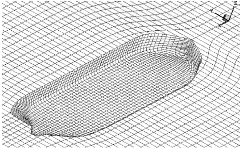
**Fig. 3.17:** A sample of panelling of the free surface and the body surface for ITU-Dawson.
