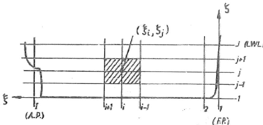
**Fig. 3.14:** Meshing of centerplane for ITU-Michell.
