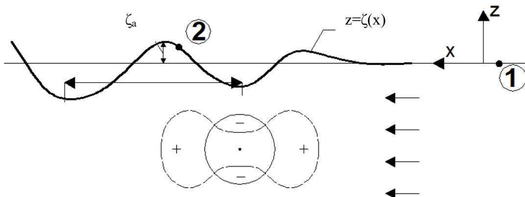
Due to the effect of free surface on the pressure distribution on the body, the result of the pressure integration over the body is other than zero and gives the wave pattern resistance in this case. Note that *Bernoulli's equation* on the free surface (streamline) gives:
