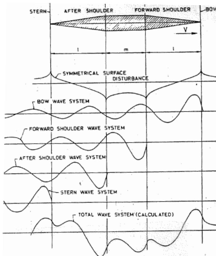
**Fig. 3.12:** Sources of wave systems on the hull and their interference (Harvald, 1991).
