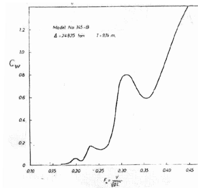
**Fig. 3.13:** Basic humps and hollows as obtained from Michell’s integral.
