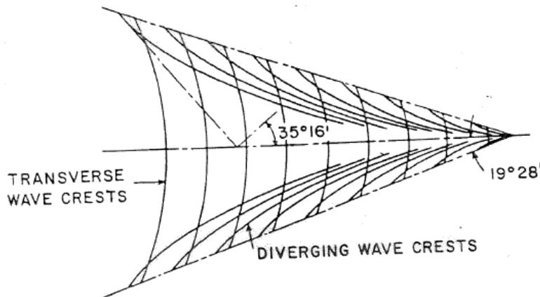
**Fig. 3.10:** Ship-wave system as obtained from Kelvin's analysis (Newman, 1980).
