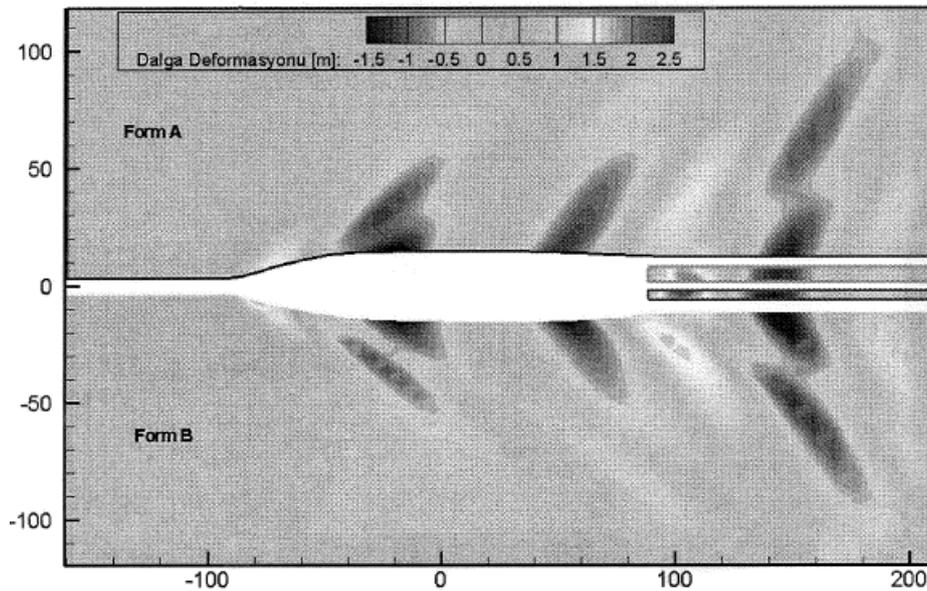
**Fig. 3.18:** Wave systems of two hull forms as computed by ITU-Dawson
