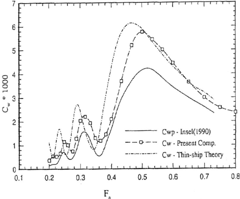
**Fig. 3.16:** Comparison of wave resistance coefficients.
