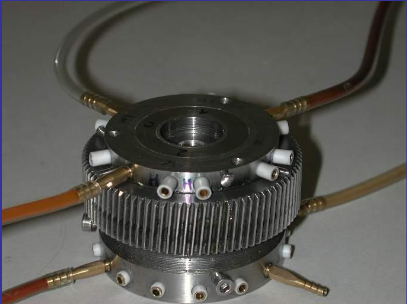
A diamond-anvil-cell device for achieving very high experimental pressures. The pipes are for the water of the cooling system.
