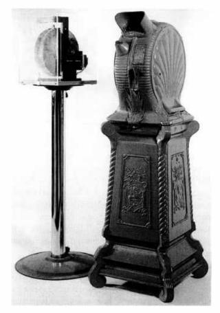
**1.12** At the right, a Mutoscope, a penny-in-the-slot machine with a crank that turned a drum containing a series of photographs. The stand at the left shows the circular arrangement of the cards, each of which flipped down and was briefly held still to create the illusion of movement.
