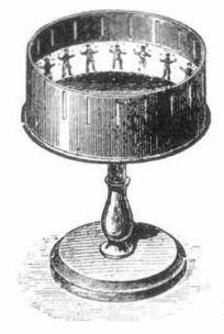
**1.2** Looking through the slots in a revolving Zoetrope, the viewer receives an impression of movement.
