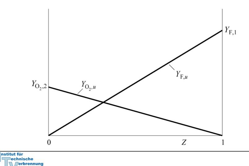
If  $Z < Z_{st}$  fuel is deficient and the mixture is called fuel lean.
