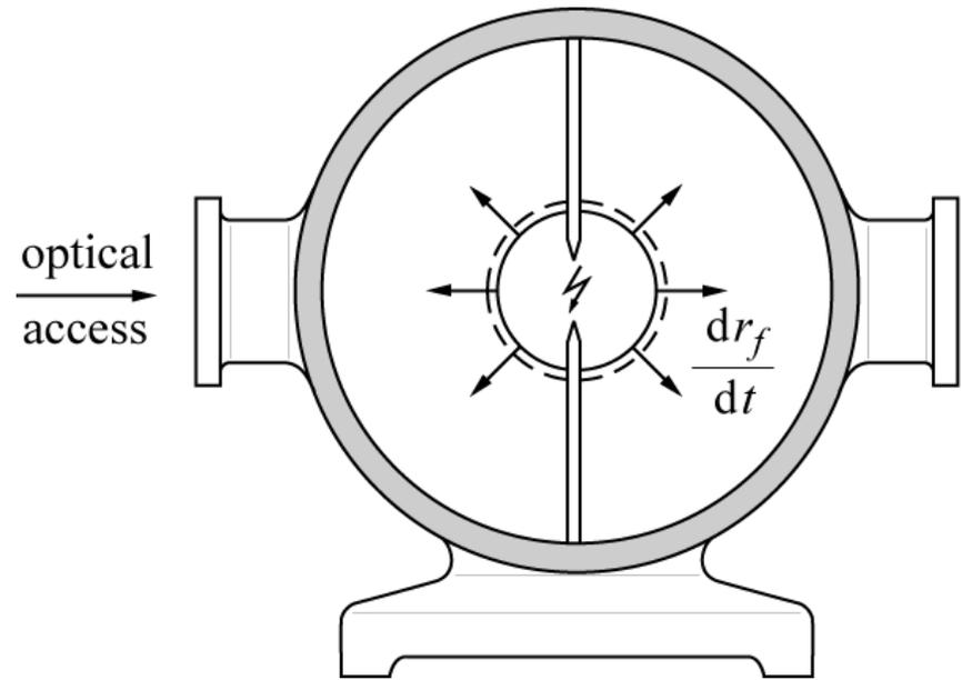
Spherical propagation of a flame then takes place which may optically be detected through quartz windows and the flame propagation velocity  $dr_f/dt$  may be recorded.
