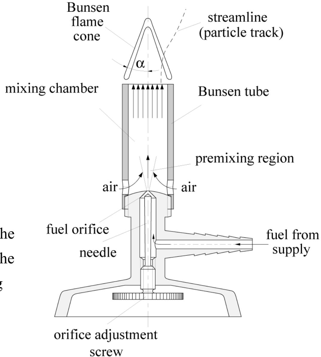
The mixing chamber must be long enough to generate a premixed gas issuing from the Bunsen tube into the surroundings.
