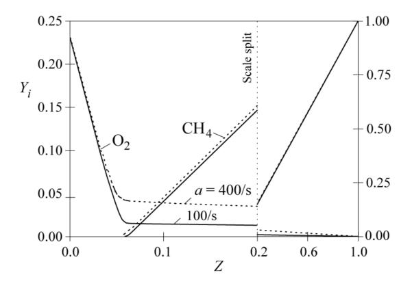
The oxygen leakage increases as extinction is approached.
