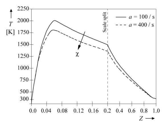
The second value of the strain rate corresponds to a condition close to extinction. It is seen that the temperature in the reaction zone decreases
