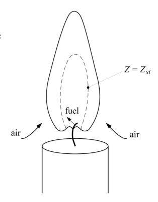
To leading order one obtains the adiabatic flame temperature which is a function of mixture fraction only.
