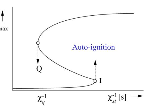
hot air leads to continuously decreasing mixture fraction gradients and therefore to decreasing scalar dissipation rates.
