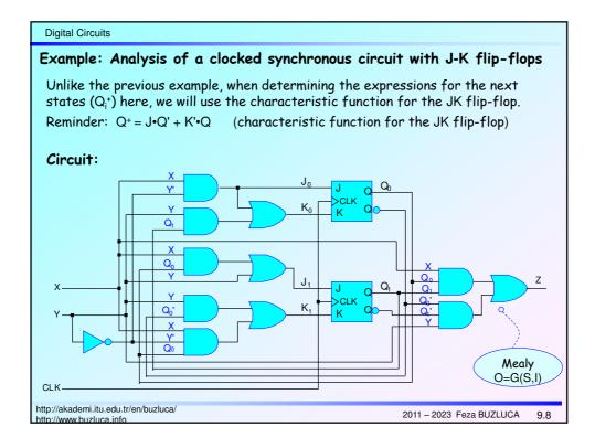
1. Determine the F function that drives the inputs of the flip-flops:
