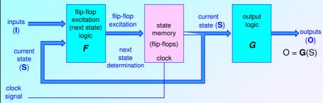
Most sequential circuits can be designed using either one of these models (Mealy or Moore).
