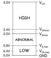
$V_{\text{OHmin}}$ : The minimum output voltage produced in the HIGH state.
