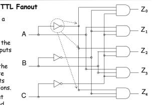
Fanout must be examined for both possible output states, HIGH and LOW.
