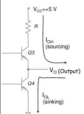
• Output is "0" (LOW):  $Q_4$  is ON,  $Q_3$  is OFF. In this case, the current  $I_{OL}$  flows into the output. The output is said to be sinking current.
