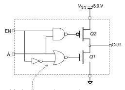
To simplify the diagram, the internal NAND, NOR, and NOT functions are represented by their own symbols rather than by their constituent transistors. These elements actually consist of 10 transistors.
