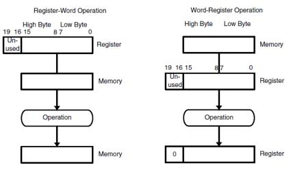
The following figure illustrates the manipulation of an address (20 bits) using the suffix .A.
