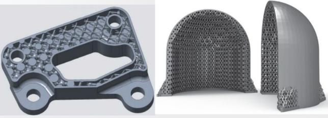
Two additively manufactured Ti64 parts built in two orientations with supports auto-generated by exaSIM
