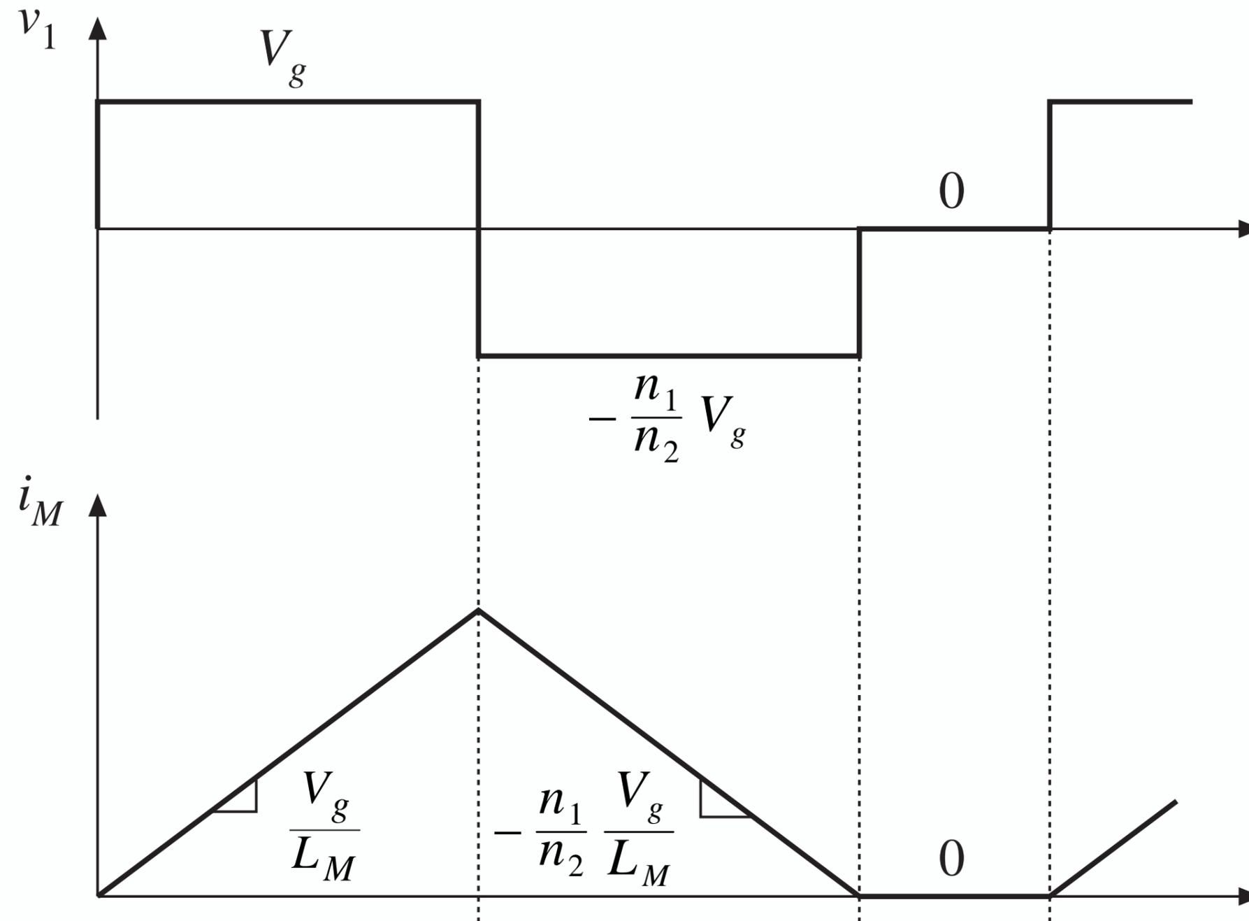
$$\langle v_1 \rangle = D(V_g) + D_2\left(-V_g n_1/n_2\right) + D_3(0) = 0$$
