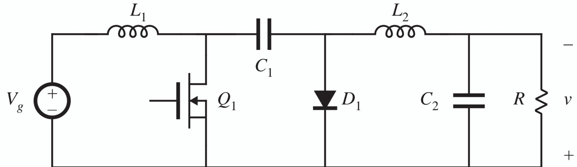
*Split capacitor  $C_1$  into series capacitors  $C_{1a}$  and  $C_{1b}$*
