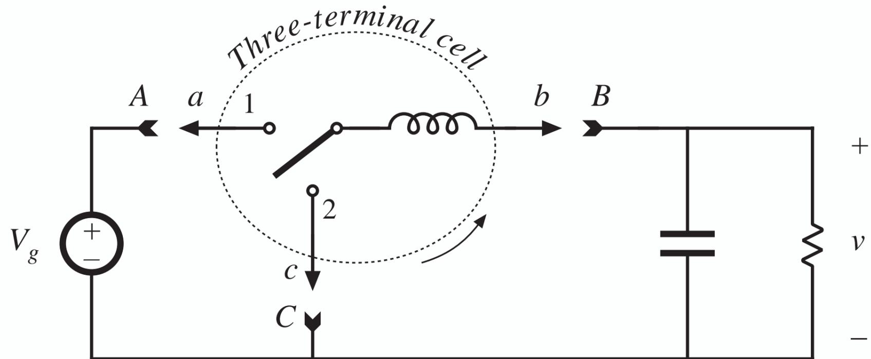
Three-terminal cell can be connected between source and load in three nontrivial distinct ways:
