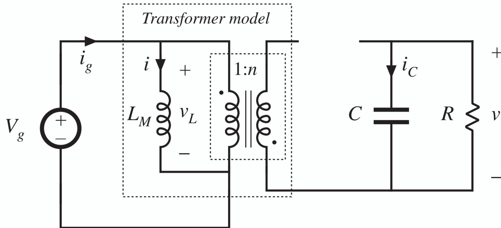
$$\begin{aligned}v_L &= V_g \\i_C &= -\frac{v}{R} \\i_g &= i\end{aligned}$$
