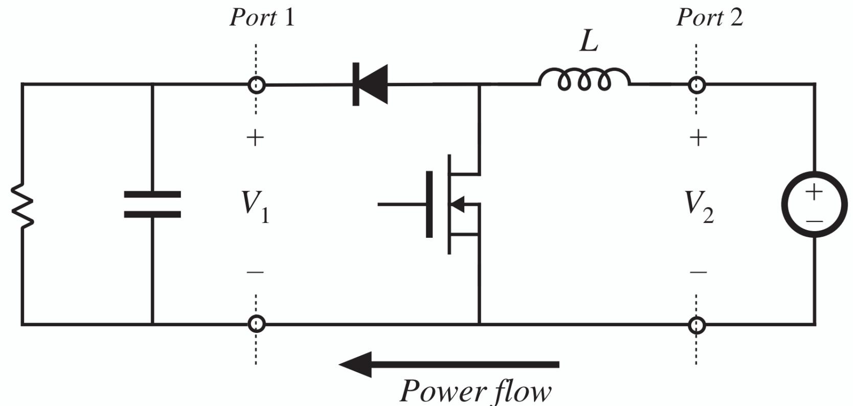
$$V_1 = \frac{1}{D'} V_2$$
