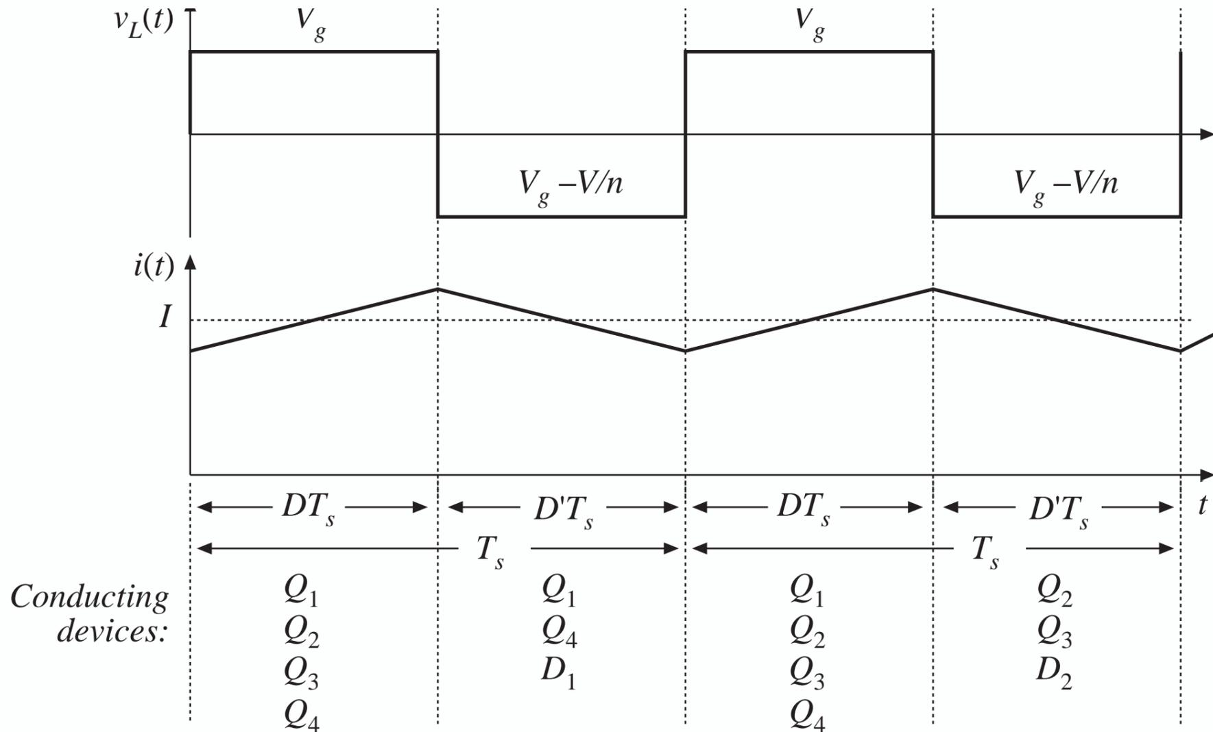
Application of volt-second balance to inductor voltage waveform:
