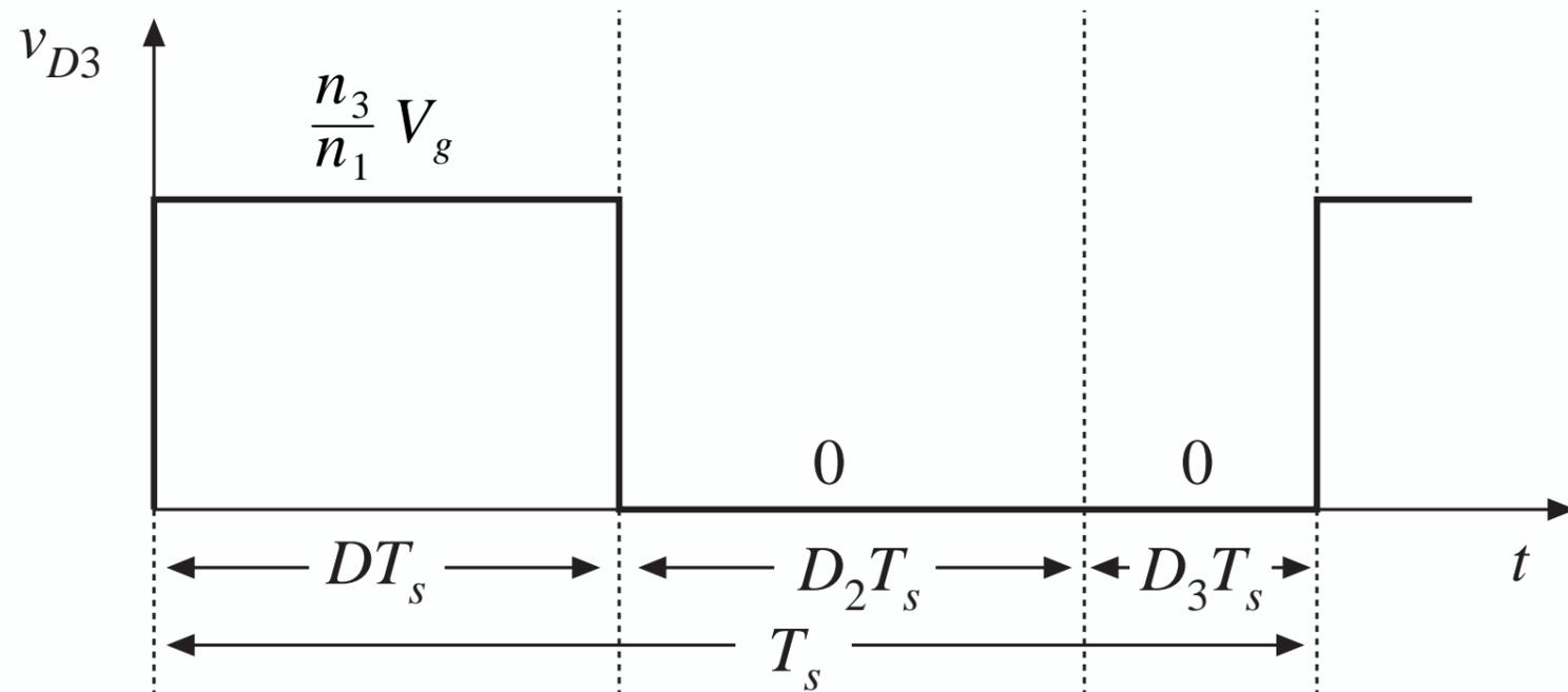
$$\langle v_{D3} \rangle = V = \frac{n_3}{n_1} D V_g$$
