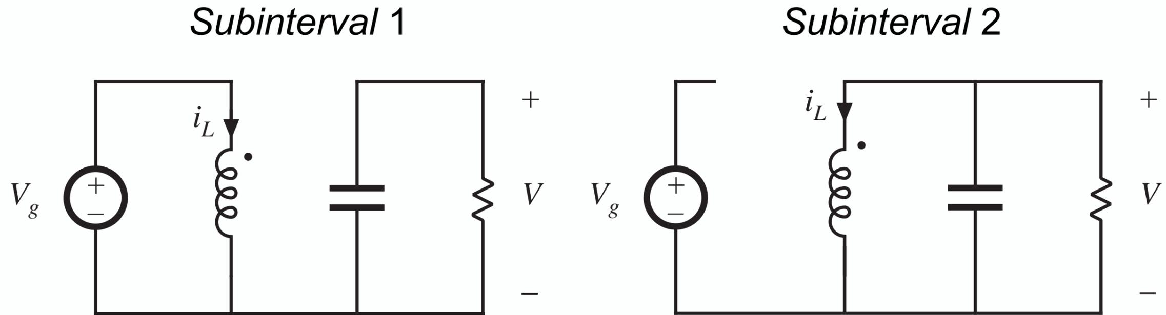
One side of inductor always connected to ground
