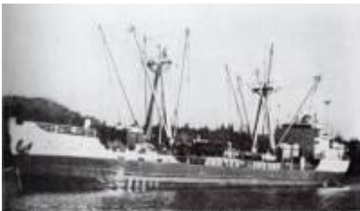
White Pass & Yukon claimed the Clifford J. Rogers was the first ship specifically designed as a container vessel. The container measured 7' x 4' x 6'.
