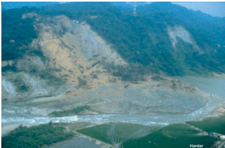
**Fig 10.1** A large landslide temporarily blocked a river following the 1999 Chi-Chi earthquake in Taiwan. (UC Davis – <https://research.engineering.ucdavis.edu/gpa/landslides/earthquake-induced-landslides/>)
