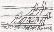
Fig. 2. Method of thatching
