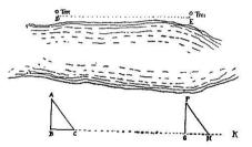
To measure the space between two distant objects, D and E. Line A B on one, then move this rightangled triangle until F G is lined on the other, with B G in line with G H. B G equals the space between D and E then.
