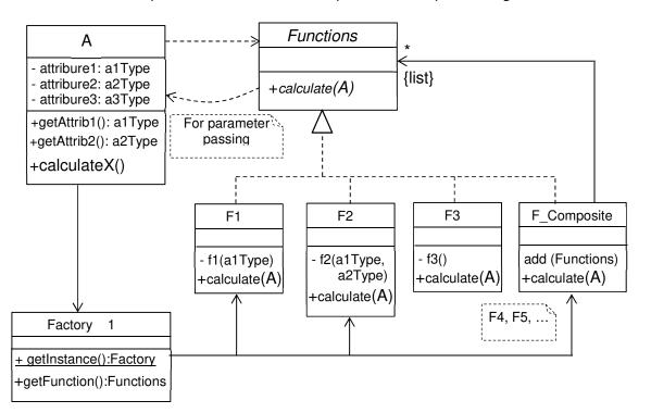
**Note:** The factory can create an object of F\_Composite and can add atomic functions into its list. This solution is flexible, because the factory can create composite objects that have different functions in their lists. It is also possible to change the list in run time.
