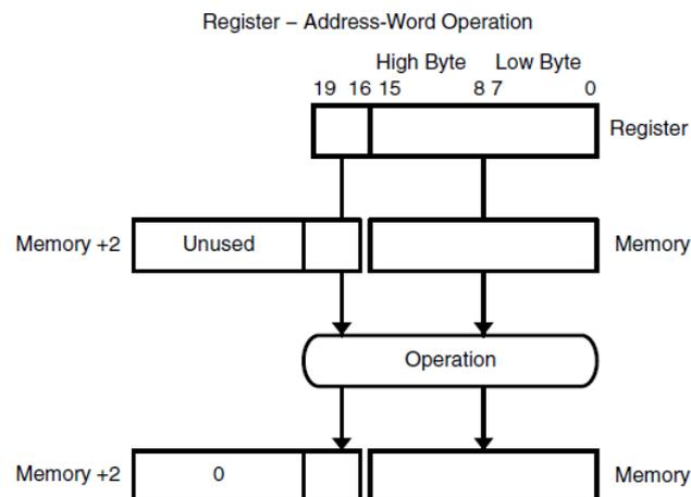
Figure 4-9. Example: Address-Word - Register operation.
