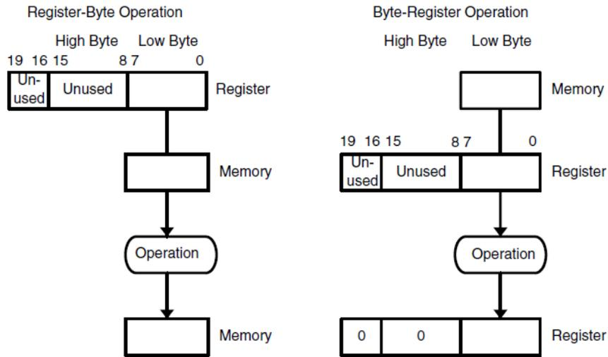
The following figure illustrates the handling of a word (16-bit) using the suffix .w.
