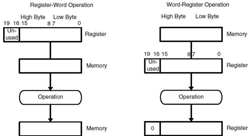
The following figure illustrates the manipulation of an address (20 bits) using the suffix .A.
