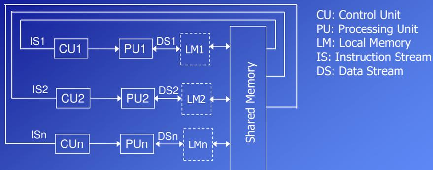
A set of processors simultaneously execute different instruction sequences on different data sets.
