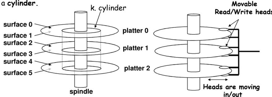
Capacity = (bytes/sector) × (avg. sectors/track) × (tracks/surface) × (surfaces/platter) × (platters/disk)
