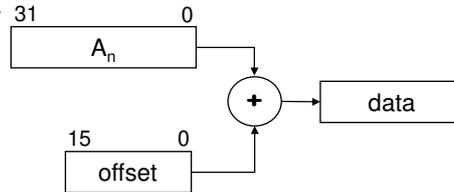
**4e. Address Register Indirect with Index and Offset**
