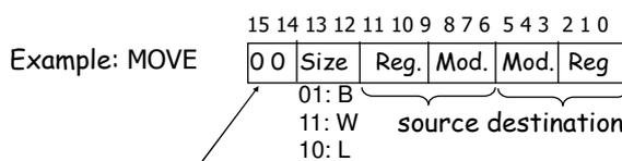
The instruction is not decoded based on just this field; the whole opword is used.
