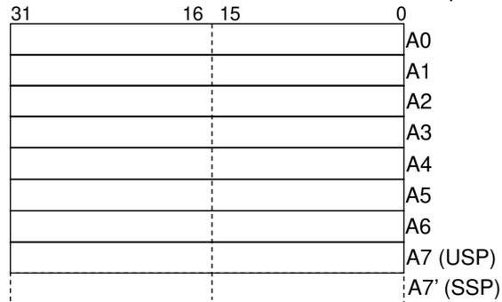
Since the address bus is 24 bits wide, only the first 24 bits of the data in an address register is used.
