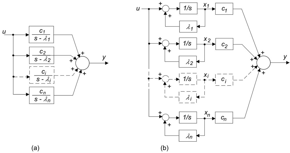
Figure 3: Diagonal form for a system with distinct eigenvalues (a) derived from partial fraction expansion of the transfer function, and (b) the block diagram for the equivalent state equations.
