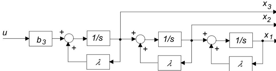
Figure 1: Block diagram of a third-order Jordan block
