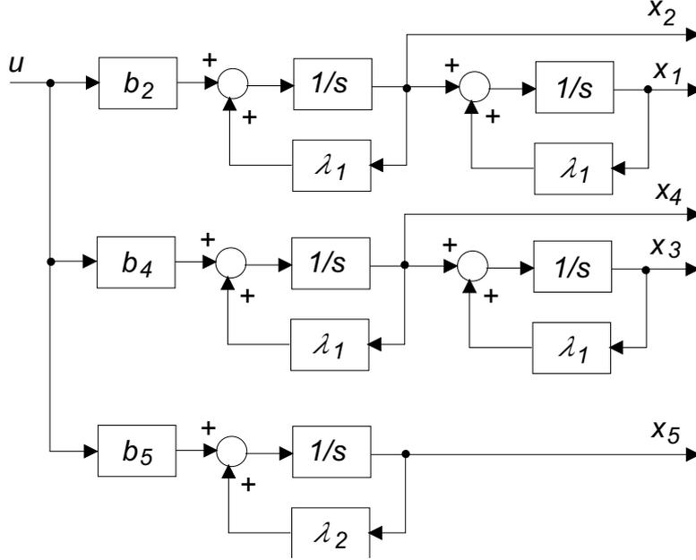
Figure 2: Block diagram of the fifth-order system with an eigenvalue of multiplicity four, and two linearly independent eigenvectors, described by Eq. (5).
