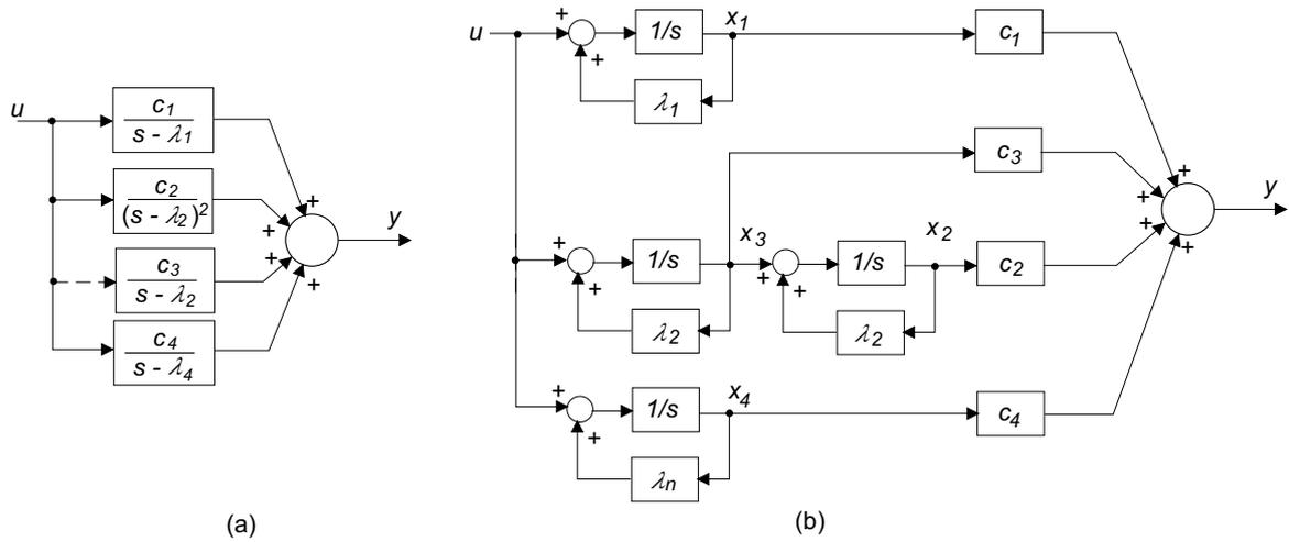
Figure 4: Diagonal form of a system with a repeated eigenvalue: (a) the block diagram from the partial fraction expansion of the transfer function, and (b) the block diagram of the equivalent Jordan form state equations.
