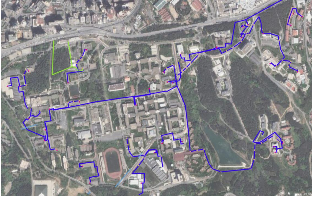
Figure 3.5 : General View of Fiber Cable Layer.
