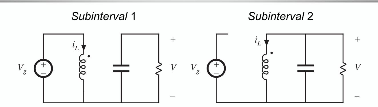
One side of inductor always connected to ground — hence, only one SPDT switch needed:
