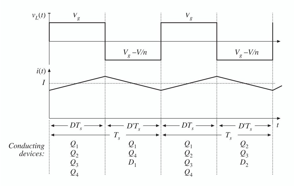
Application of volt-second balance to inductor voltage waveform:
