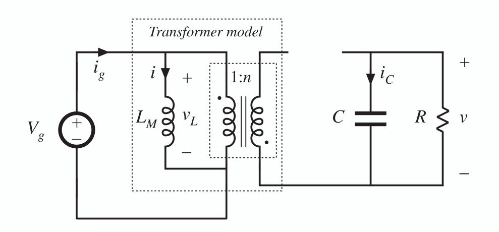
$$egin{aligned} v_L &= V_g \ i_C &= -rac{v}{R} \ i_g &= i \end{aligned}$$
