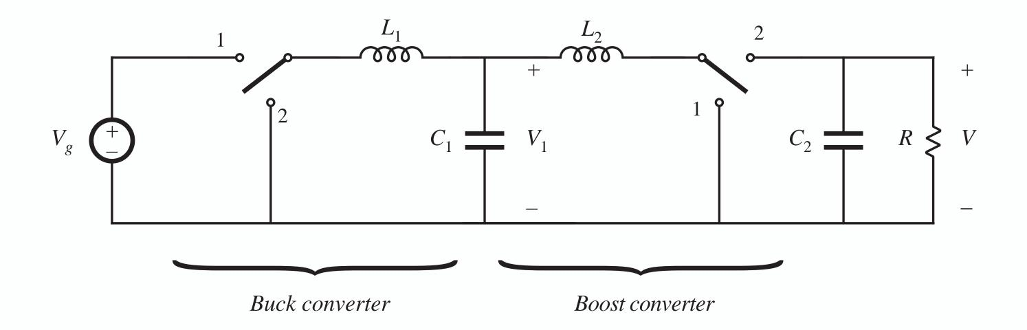
$$\frac{\frac{V_1}{V_g} = D}{\frac{V}{V_1} = \frac{1}{1 - D}}$$
