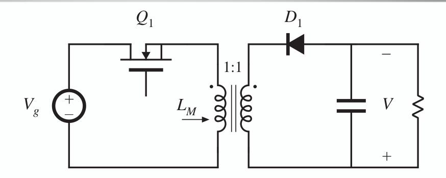
Flyback converter having a 1:n turns ratio and positive output:
