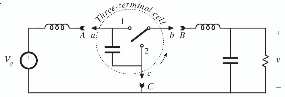
Three-terminal cell can be connected between source and load in three nontrivial distinct ways:
