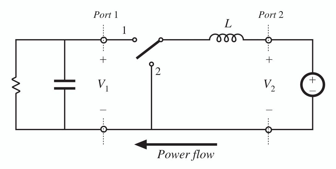
$$V_2 = DV_1 \qquad \qquad V_1 = \frac{1}{D} V_2$$
