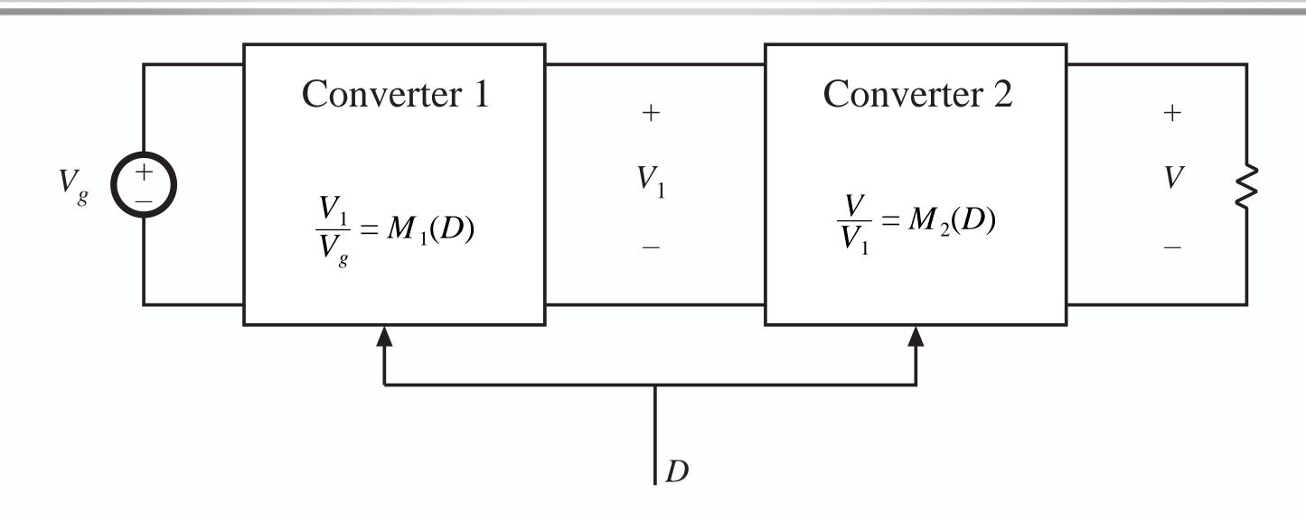
$$V_{1} = M_{1}(D)V_{g}$$
