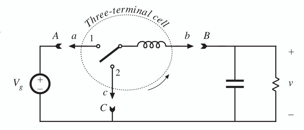
Three-terminal cell can be connected between source and load in three nontrivial distinct ways:
