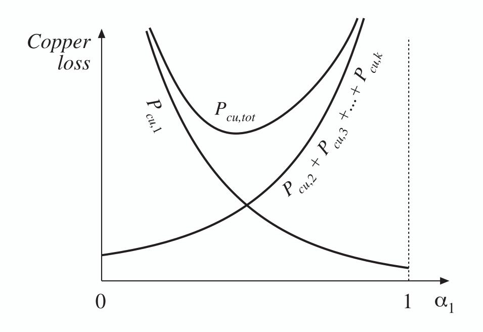
For  $\alpha_1 = 0$ : wire of winding 1 has zero area.  $P_{cu,1}$  tends to infinity
