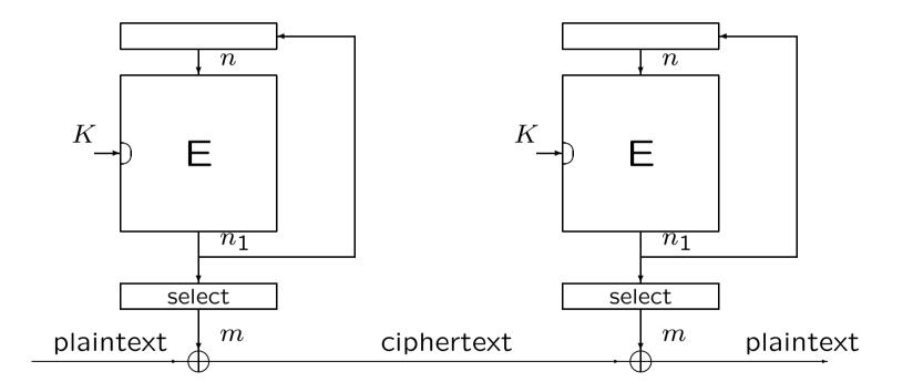
$n = \text{block length}, n_1 = \# \text{ of feedback bits}$  $n_1 < n, m = \# \text{ of selected key stream bits}$
