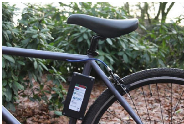
Fig. 1 Sensor unit developed by CoSynth used in the ECOSense project. Source: University of Oldenburg
