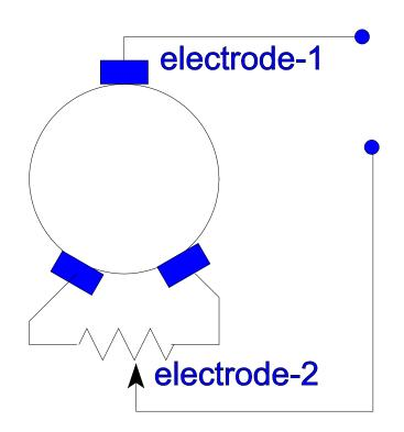
The variable resistance adjusts the direction of the field till it is parallel to the external field
