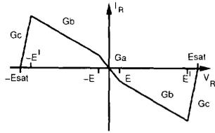
Fig. 19. Every physically realizable nonlinear resistor  $N_R$  is eventually passive—the outermost segments (while not necessarily linear as shown here) must lie completely within the first and third quadrants of the  $V_R$ - $I_R$  plane for sufficiently large  $|V_R|$  and  $|I_R|$ .
