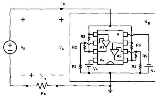
Fig. 21. The DP characteristic of Chua diode  $N_R$  can be measured by applying a triangular voltage waveform  $V_S$  to the series combination of  $N_R$  and a small current-sensing resistor  $R_S$ . Plot  $-V_{I_R} (\propto I_R)$  versus  $V_R$ . The eight-pin dual op amp package is shown from above in schematic form. The reference end of the package is indicated by a dot or a semicircle (shown here).
