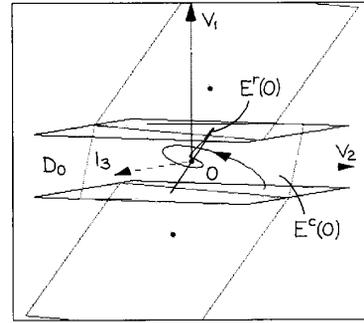
Fig. 5. Dynamics of the  $D_0$  region. A trajectory starting slightly above the stable complex eigenplane  $E^c(0)$  spirals toward the origin along this plane and is repelled close to 0 in the direction of the unstable eigenvector  $E^r(0)$ .
