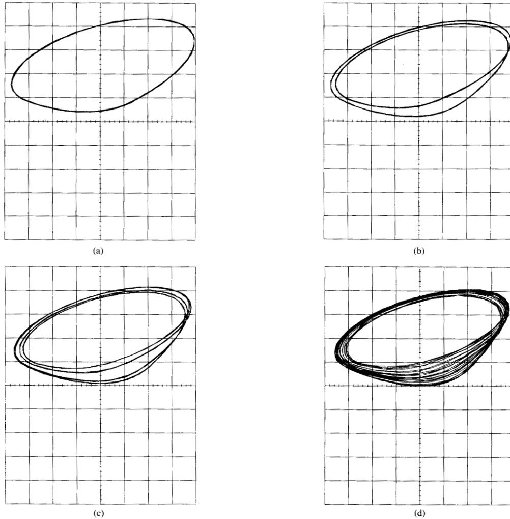
Fig. 23. Typical experimental bifurcation sequence in Chua's circuit (component values as in Table I) recorded by using a Hitachi VC-6025 Digital Storage Oscilloscope. Horizontal axis  $V_2$  (a)–(h) 200mV/div, (i) 2V/div; vertical axis  $V_1$  (a)–(h) 1V/div, (i) 2V/div. (a)  $R = 1.83k\Omega$ , period 1; (b)  $R = 1.82k\Omega$ , period 2; (c)  $R = 1.81k\Omega$ , period 4; (d)  $R = 1.80k\Omega$ , Spiral-Chua attractor.
