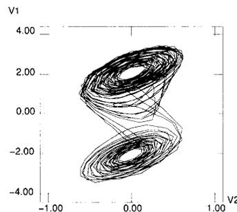
Fig. 25. SPICE 3e2 simulation of Fig. 18 using the input deck shown in Fig. 24 yields this double-scroll Chua attractor. Horizontal axis  $V_2$  (V); vertical axis  $V_1$  (V). The jaggedness of the trajectory results from the large timestep chosen by SPICE's integration routine when using its default accuracy settings.
