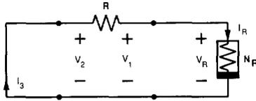
Fig. 8. dc equivalent circuit of Fig. 2 obtained by short-circuiting the inductor  $L$  and open-circuiting capacitors  $C_1$  and  $C_2$ .
