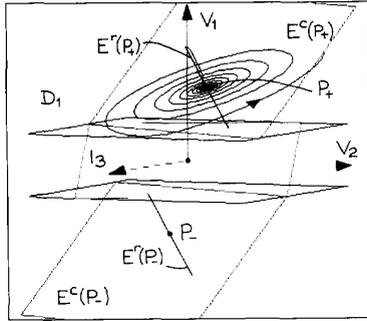
Fig. 7. Dynamics of the  $D_1$  region. A trajectory starting above the unstable complex eigenplane  $E^c(P_+)$  close to the eigenvector  $E^r(P_+)$  moves toward the plane and spirals away from  $P_+$  along  $E^c(P_+)$ . By symmetry, the  $D_{-1}$  region has equivalent dynamics.
