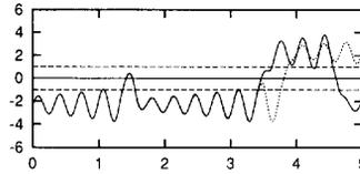
Fig. 14. Sensitive dependence on initial conditions. Two time waveforms  $V_1(t)$  from Chua's oscillator with  $G = 550\mu S$ , starting from  $(I_3, V_2, V_1) = (1.810\text{mA}, 222.014\text{mV}, -2.286\text{V})$  [solid line] and  $(I_3, V_2, V_1) = (1.810\text{mA}, 222.000\text{mV}, -2.286\text{V})$  [dashed line]. Note that the trajectories diverge within 5 ms. Horizontal axis:  $t$  (ms); Vertical axis:  $V_1$  (V). Compare with Fig. 13.
