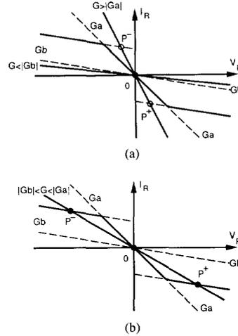
Fig. 9. dc equilibrium points of Fig. 2 may be determined graphically by intersecting the load line  $I_R = -GV_R$  with the DP characteristic of  $N_R$ . (a) If  $G > |G_a|$  or  $G < |G_b|$ , the circuit has a unique equilibrium point at the origin ( $P_-$  and  $P_+$  are virtual equilibria in this case). (b) When  $|G_b| < G < |G_a|$ , the circuit has three equilibrium points at  $P_-, 0$ , and  $P_+$ .
