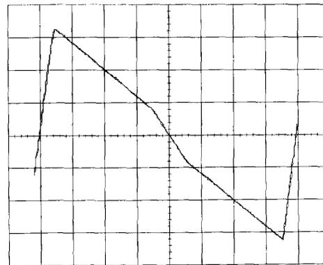
Fig. 22. Measured  $v$ - $i$  characteristic of the Chua diode in Fig. 18.  $V_S$  is a triangular waveform with zero DC offset, amplitude 15V peak-to-peak, and frequency 30 Hz. Horizontal axis:  $V_R$  (2V/div); Vertical axis:  $-V_{I_R}$  (100mV/div).
