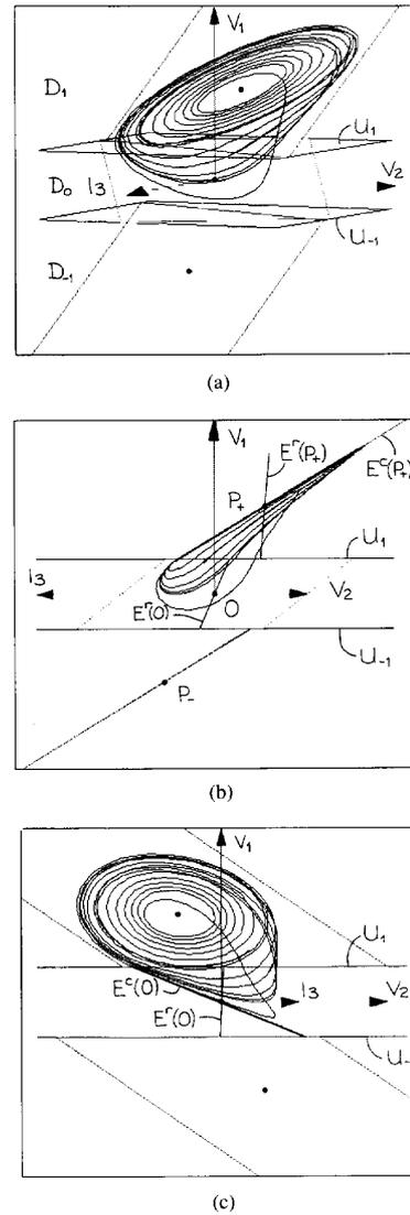
Fig. 12. Three views of a simulated Spiral-Chua attractor in Chua's oscillator with  $G = 550\mu S$ . (a) Reference view (compare with Figs. 10 and 11). (b) View along the edge of the outer complex eigenplanes  $E^c(P_+)$  and  $E^c(P_-)$ ; note how the trajectory in  $D_1$  is flattened onto  $E^c(P_+)$ . (c) View along the edge of the complex eigenplane  $E^c(0)$ ; trajectories cannot cross this plane.
