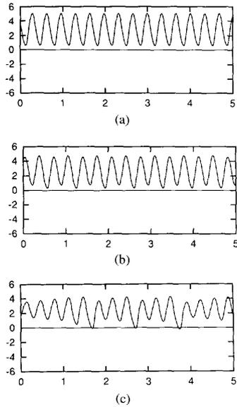
Fig. 15. Simulated time waveforms  $V_1(t)$  from Chua's oscillator with (a)  $G = 530\mu\text{S}$  (period 1 limit cycle); (b)  $G = 537\mu\text{S}$  (period 2 limit cycle); (c)  $G = 550\mu\text{S}$  (Spiral-Chua chaotic attractor). Horizontal axis:  $t$  (ms); Vertical axis:  $V_1$  (V). Compare with Figs. 10(b), 10(c), and 12, respectively.
