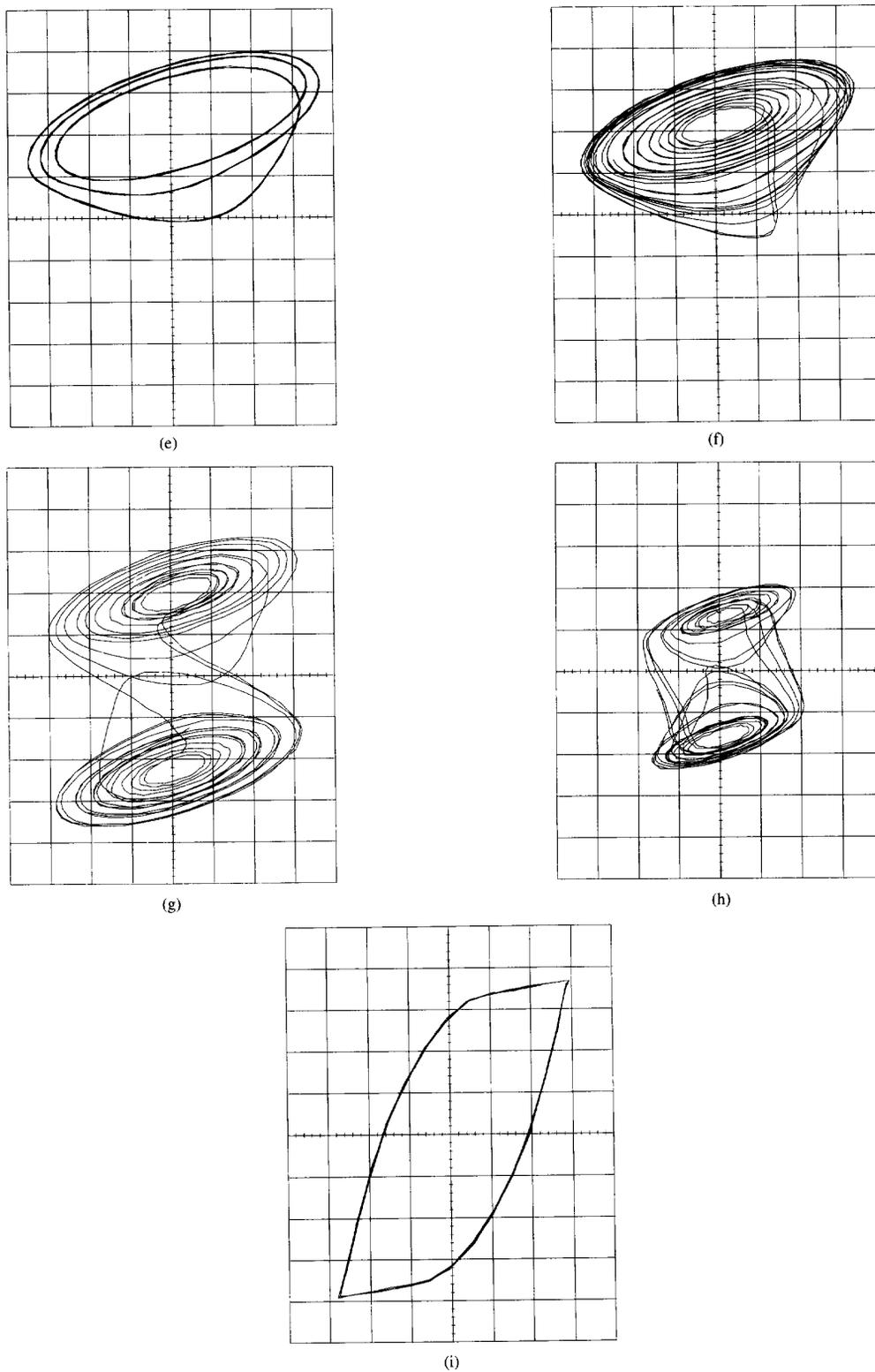
Fig. 23 (continued). (e)  $R = 1.797k\Omega$ , period 3 window; (f)  $R = 1.76k\Omega$ , Spiral-Chua attractor; (g)  $R = 1.73k\Omega$ , double-scroll Chua attractor; (h)  $R = 1.52k\Omega$ , double-scroll Chua attractor; (i)  $R = 1.42k\Omega$ , large limit cycle corresponding to the outer segments of the Chua diode's DP characteristic.
