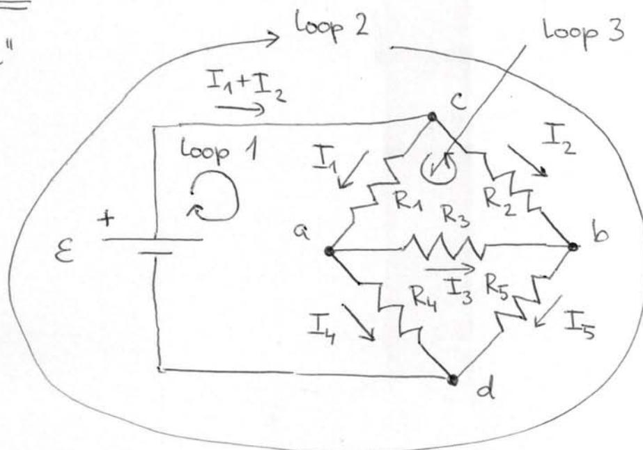
$$R_1 = R_2 = R_3 = R_4 = 1\Omega$$
