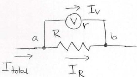
$$I_{total} = I_R + I_V = \frac{V_{ab}}{R} + \frac{V_{ab}}{r} =$$
