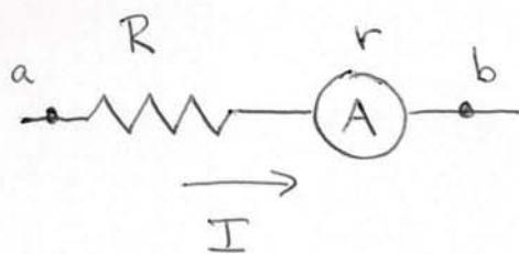
$$I = \frac{V_{ab}}{R+r} \Rightarrow r \ll R \text{ required}$$
