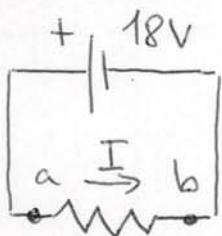
$$V_{ab} = \mathcal{E} \Rightarrow I = \frac{V_{ab}}{R_{123}} = \frac{\mathcal{E}}{R_{123}} = 3A$$
