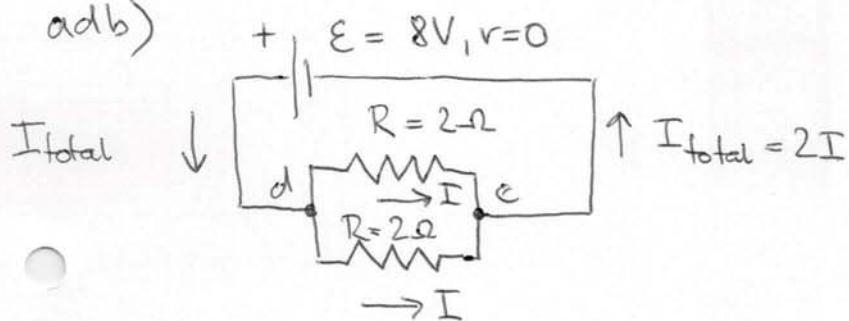
$$\frac{1}{R_{\text{eq}}} = \frac{2}{R} \Rightarrow R_{\text{eq}} = \frac{R}{2} = \underline{\underline{1\Omega}}$$
