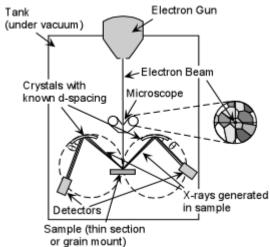
Electrons striking the small area of the sample produce X-rays with wavelengths characteristic of the elements in the sample. The spectrometers consist of curved crystals of known d-spacing. These crystals diffract X-rays of each element into the detectors at the diffraction angle  $\theta$ . Several elements can be measured at once, then the spectrometers are set to new angles to measure the X-ray intensities of several more elements.
