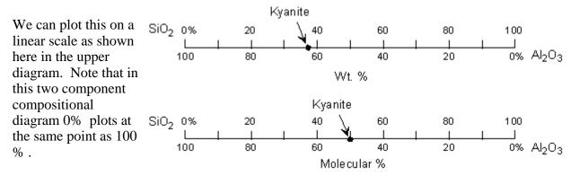
We could divide each of these weight percentages by the molecular weight of each of the oxides and recalculate in the analysis in terms of molecular %. But the chemical formula of Kyanite -  $Al_2SiO_5$  - tells us that kyanite is made up of  $1Al_2O_3 + 1SiO_2$ . So in molecular percent 50% of kyanite is  $Al_2O_3$  and 50% is  $SiO_2$ , as shown in the lower diagram above.
