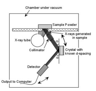
Intensities of characteristic X-rays for each element of interest are determined by rotating the crystal and detector to the angle  $\theta$  required for diffraction of the characteristic X-ray wavelength. X-ray intensities are then measured for each element in the unknown and for each element in a standard that has known concentrations. The following equations are then used to determine the concentration of each element in the unknown:
