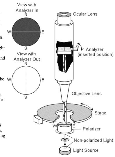
If the analyzer is out, so that it is not in the light path, then the polarized light will be transmitted through the ocular lens.
