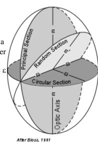
Thus, the uniaxial indicatrix is seen to be an ellipsoid of revolution. Such an ellipsoid of revolution would be swept out by rotating the ellipse of the principal section by 180°. Note that there are an infinite number of principal sections that would cut the indicatrix vertically.
