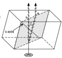
Since the angle of incidence of the light is  $0^{\circ}$ , both rays should not be refracted when entering the crystal according to Snell's Law, but the e-ray violates this law because it's angle of refraction is not  $0^{\circ}$ , but is r, as shown in the figure. Note that the vibration directions of the e-ray and the o-ray are perpendicular to each other. These directions are referred to as the *privileged directions* in the crystal.
