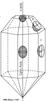
• If the crystal is mounted on the stage such that the c-axis or optic axis is neither parallel to or perpendicular to the stage, we can move the indicatrix to some random face that is not parallel to or perpendicular to the c-axis (such as face b) and see that the light will be broken into two perpendicular rays, one vibrating parallel to the  $\omega$  direction and the other vibrating perpendicular to an  $\epsilon'$  direction. Thus we will see one of the random sections of the indicatrix.
