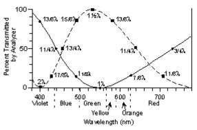
If the crystal produces a retardation of 800 nm, the dashed curve would be obtained. This curve shows little transmission of the violet and red wavelengths, and partial to full transmission of the green, yellow, and orange wavelengths. Thus the crystal will have a greenish interference color.
