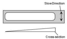
The wedge, like all compensators usually has its slow direction clearly marked, and is inserted into the microscope tube such that slow direction in the compensator is at a  $45^{\circ}$  angle to the polarizing direction. You will see a quartz wedge in the lab, but the microscopes we use do not have a slot that accommodates these older wedges. In today's economy, quartz wedges are too expensive to equip student microscopes with them.
