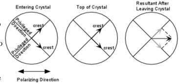
At the top of the crystal, the waves are still in phase (i.e. their path difference is  $n\lambda$ ), and thus their wave crests are at the same positions as when they entered the crystal. These waves are then resolved into a single polarized waved that is vibrating parallel to the polarizer. Such a wave will be extinguished by the analyzer.
