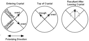
This time, the resultant wave produced by recombination of the two polarized waves after leaving the crystal will have a resultant wave vibrating perpendicular to the polarizer (parallel to the analyzer), and thus this light will pass the analyzer. The color will be that of the monochromatic light that entered the crystal from below. Again, this will occur if the path difference is equal to an odd multiple of  $\frac{1}{2}\lambda$ .
