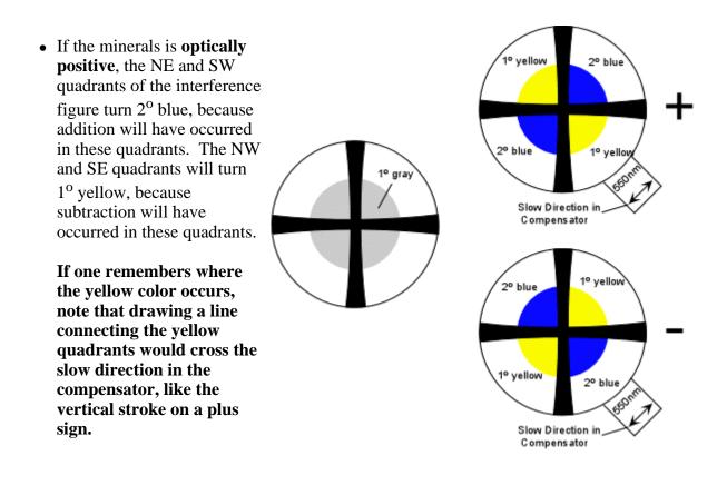
• If the minerals is **optically negative**, the NE and SW quadrants of the interference figure turn 1° yellow, because subtraction will have occurred in these quadrants. The NW and SE quadrants will turn 2° blue, because addition will have occurred in these quadrants.
