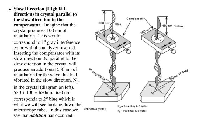
More importantly, if an area on the crystal that was 1<sup>o</sup> gray turns blue on insertion of the compensator, we know the direction in the crystal parallel to the slow direction in the compensator is the slow direction or higher R.I. direction.
