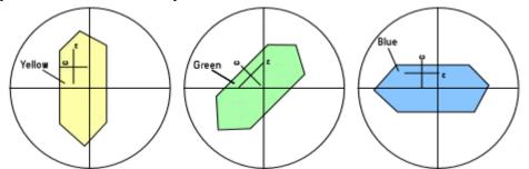
When the  $\varepsilon$  direction is parallel to the polarizer only light vibrating in the in the  $\varepsilon$  direction will pass through the crystal and it will show the blue absorption color in the case illustrated.
