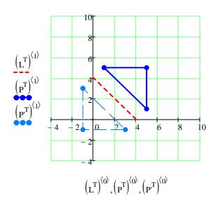
**5.** (**30** points) A Bezier curve p(u) is defined by control points in Fig.3. Use the iterative (recursive subdivision, lineer interpolation, deCasteljau, DeBoor) algorithm to compute: p(1/2).
